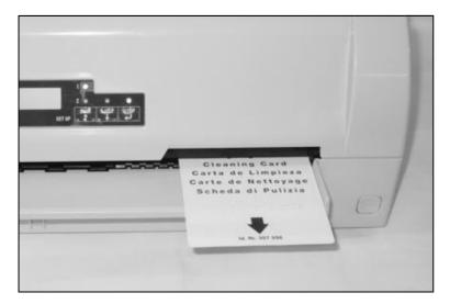
Insert the special MSR-H cleaning sheet at the right side of the printer.
