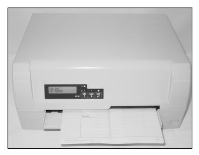
After the passbook is printed, it should be automatically ejected from the printer and released for removal. If the passbook has not successfully ejected from the printer, press the **STOP key** to to take the printer to STOP (Offline) mode: press the **STOP key** again to eject the passbook.
