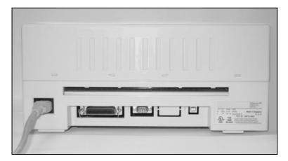
Connect the power cable to the power inlet of the printer. Connect the power cable plug to a mains socket. User Guide Installation
