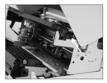
First insert the new ribbon cassette by hooking it into the rear slots of its mountings.
