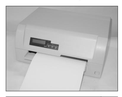
Insert the document in such a way that the right paper edge is positioned inside the area between the left side of the symbol and the right edge of the document support, so that the document alignment can grasp it securely. This is especially important for documents that are narrower than a A4 sheet.
