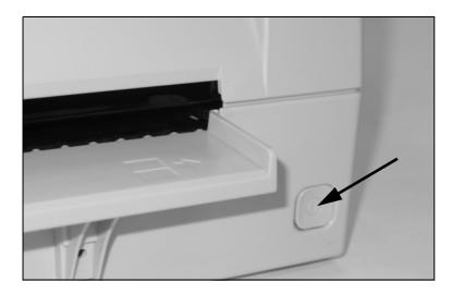
Press the power switch which is located at the front bottom right of the printer to switch on the printer.
