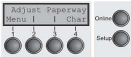
**Setup** key: Sets the printer to setup mode, in which the following settings can be selected:
