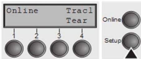
Select the **Setup** mode by pressing the **Setup** key.
