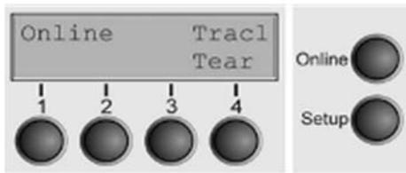
**Tear** key (4): Activates the tear function when fanfold paper is loaded.. If **Load** is displayed above this key, no paper is loaded in the printer or the printer is in park position. In this case the display switches between **Online** and **Load paper fromTrac1**. Press the key to feed paper to the printing position.
