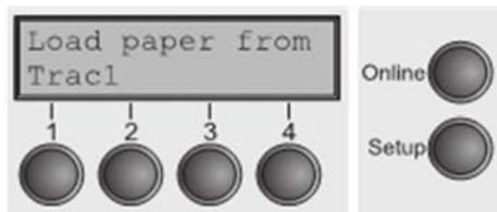
The paper is automatically loaded when the printer is in online mode and receives data from the computer.
