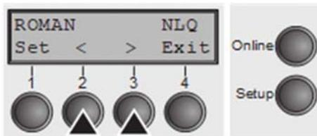
If you pressed the **Font** (1) key, use the < (2) or > (3) key to select the desired font. Confirm the selection by pressing the **Set** (1) key.
