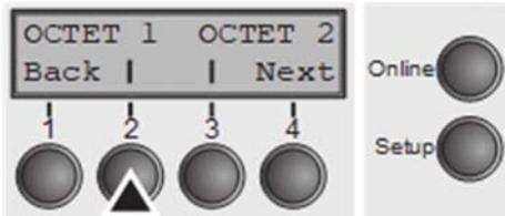
This menu level offers the possibility to set the IP address, which is divided into four digit groups (octet 1 to 4). You can activate octet 3 and 4 by pressing the **Next** (2) key.
