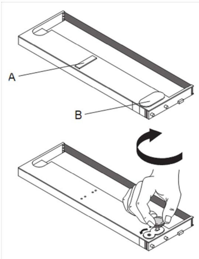
Insert the coloured ribbon tension knob into the right-hand front location of the new ribbon cassette. Turn the knob in the direction of the arrow in order to take up slack of the ribbon.
