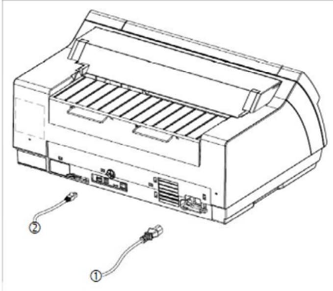
Connect the power cable (1) to the power inlet of the printer. Connect the power cable plug to a mains socket.
