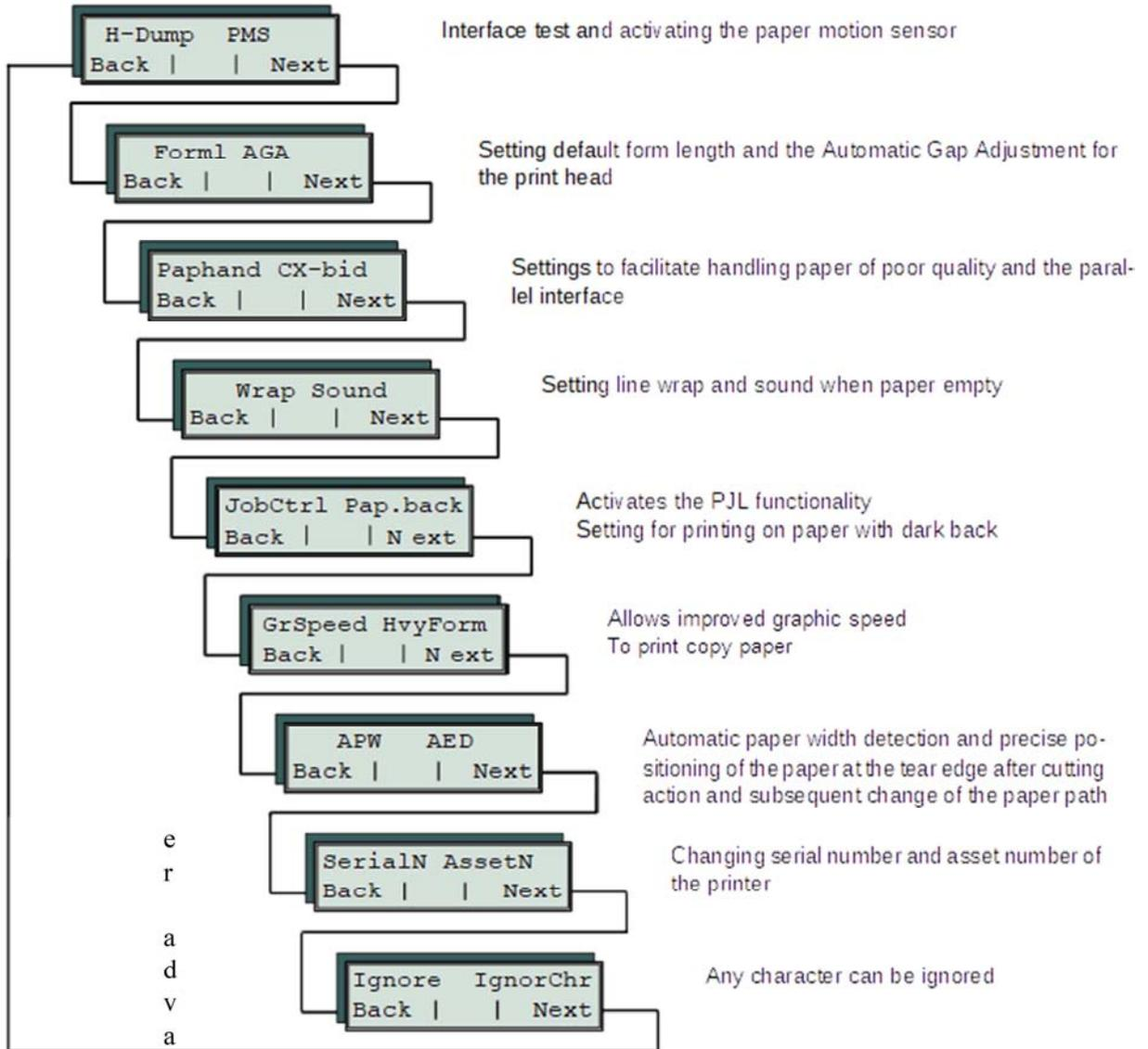
Enter advanced menu mode by pressing the key Online while switching on the printer.
